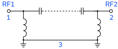
Figure 1. HFHKI-5000+ Functional Diagram
