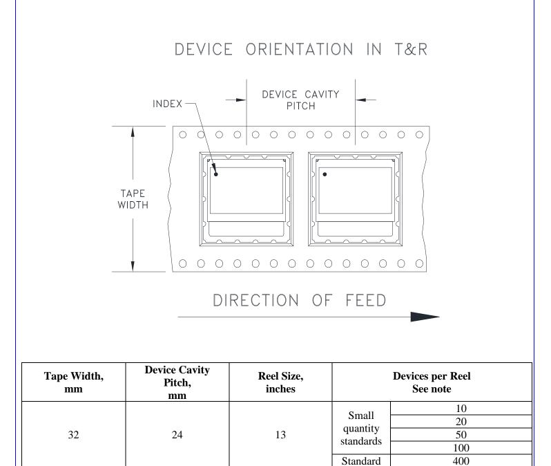
Note: Please consult individual model data sheet/dashboard to determine device per reel availability. Mini-Circuits carrier tape materials provide protection from ESD (Electro-Static Discharge) during handling and transportation. Tapes are static dissipative and comply with industry standards EIA-481/EIA-541.
