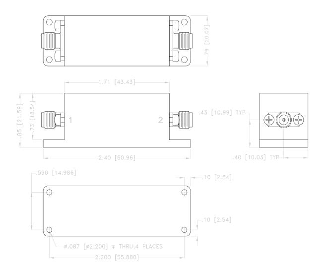
Dimensions are in inches (mm). Tolerances:  $2 \text{ Pl.} \pm .10 (2.54)$ ;  $3 \text{ Pl.} \pm .015 (0.381)$
