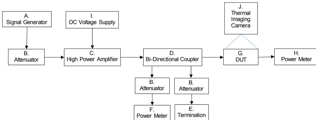
**Figure 3: LFCW Series Power Handling Test Block Diagram**
