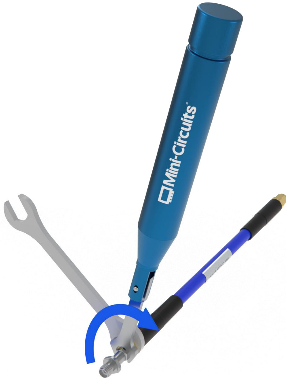
Figure 4: 1.0 mm adapter being torqued onto the end of a 1.0 mm cable with the cable connector stabilized by an open-end wrench.
