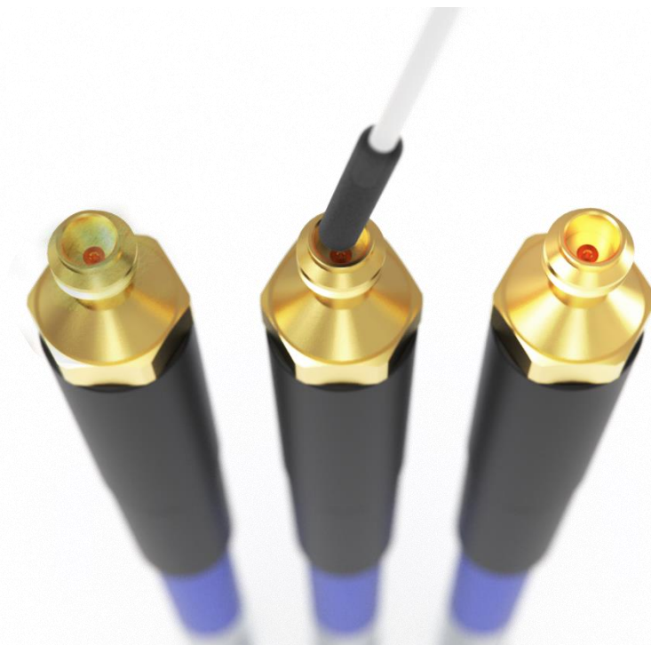
Figure 1: 1.0 mm connectors showing signs of debris (left), cleaning with a foam swab (center), and resulting clean connector (right).
