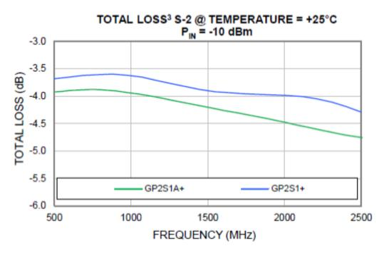
3. Total Loss = Single Path (S-1 or S-2) Insertion Loss + 3 dB Splitter Loss
