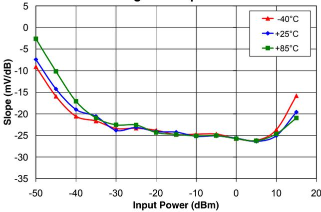
**Slope Vs Freq Over Temperature Range @ Input Power -40dBm**
