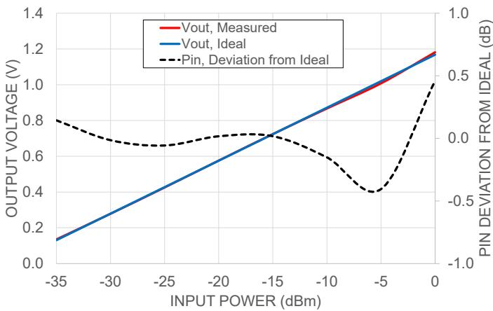
INPUT POWER DEVIATION FROM IDEAL vs INPUT POWER @ FREQUENCY 20 GHz
