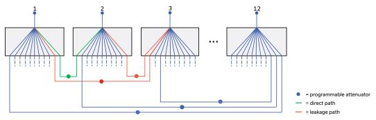
The green path in the diagram above is the direct path between ports 1 & 2. In an ideal mesh this would be the only route between these 2 ports. The insertion loss (IL) on the direct path is approximately as below, when the attenuator highlighted in green is set to 0 dB:
