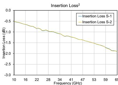
2. Insert loss is loss above theoretical loss (-3dB)
