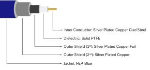
2. Cable construction drawing does not include the armored braiding
