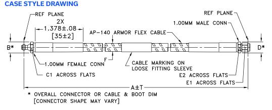
Unless Otherwise Specified dimensions are in inches [mm], Tolerances:2 Pl.±0.03[0.76]; 3 Pl. ±0.015[0.38] inches[mm]
