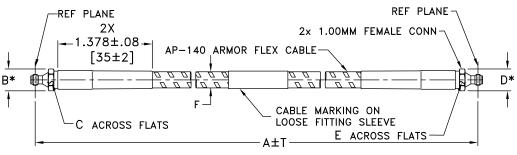
\* OVERALL CONNECTOR OR CABLE & BOOT DIM [CONNECTOR SHAPE MAY VARY]
