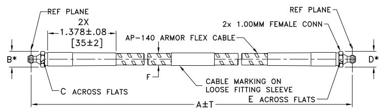
\* OVERALL CONNECTOR OR CABLE & BOOT DIM [CONNECTOR SHAPE MAY VARY]
