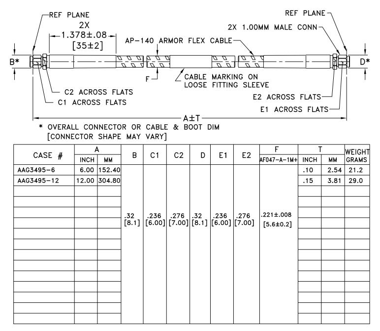
Unless Otherwise Specified dimensions are in inches [mm], Tolerances: 2 Pl.±0.03[0.76]; 3 Pl. ±0.015[0.38] inches[mm]
