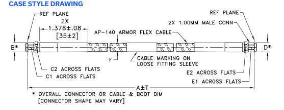
Unless Otherwise Specified dimensions are in inches [mm], Tolerances: 2 Pl.±0.03[0.76]; 3 Pl. ±0.015[0.38] inches [mm]
