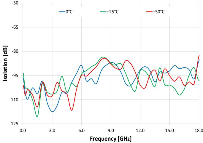
**Isolation J7 to J8 (J7 Active)**
