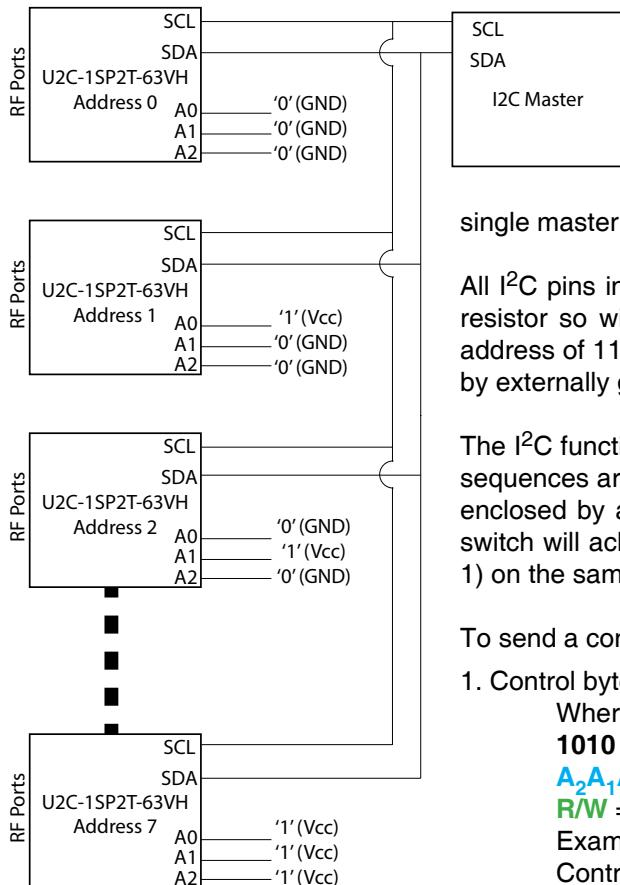
The I<sup>2</sup>C is a short-range synchronous communication protocol for simple 2-wire communication with slave devices using clock (SCL) and data (SDA) connections. The U2C-1SP2T-63VH interface also includes 3 address pins (A0, A1 and A2), allowing up to 8 switches to be controlled independently from a single master with shared SDA and SCL connections.
