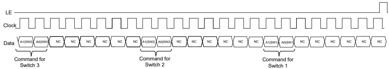
**Figure 4: Example of command for 3 switches in series**
