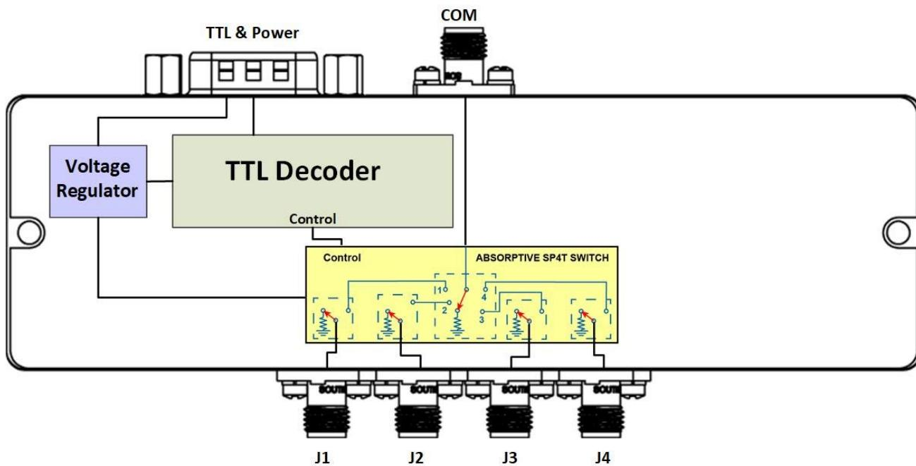
Switch functional diagram shown in disconnected state**CONNECTIONS**
