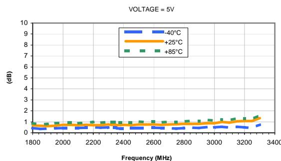
OUTPUT RETURN LOSS vs. FREQUENCY & TEMPERATURE
