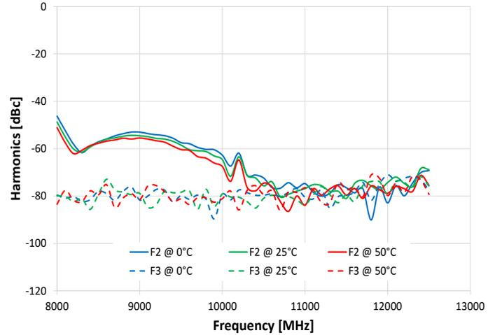
Harmonics vs. Output Frequency @ -20 dBm
