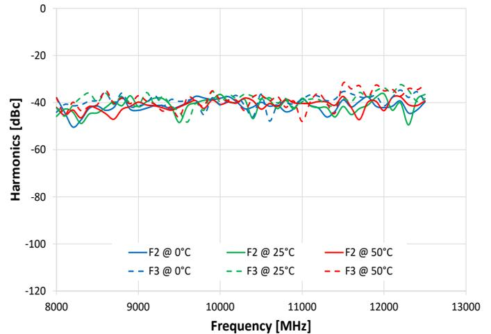
Harmonics vs. Output Frequency @ -50 dBm
