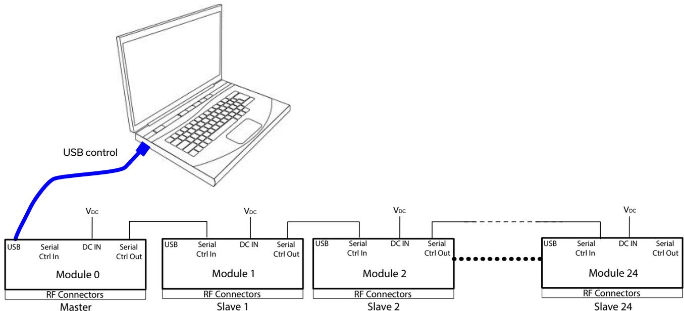
Connections between modules will be made using the serial in/out ports with the module connected to the PC act as a master and all other as slave modules. All control will be through the master module (address 0) which is the only one communicating with the PC or computer network. Serial control out port of each module should be connected to the serial control in port of the next module.
