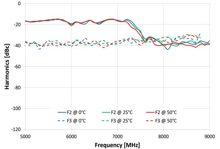
Harmonics vs. Output Frequency @ -50 dBm
