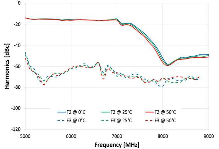
Harmonics vs. Output Frequency @ -20 dBm
