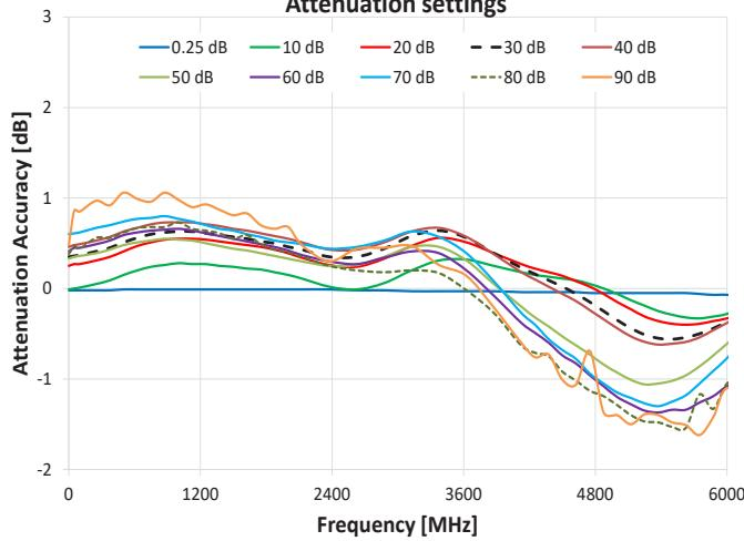
Attenuation Accuracy @ 50°C vs. Frequency over
