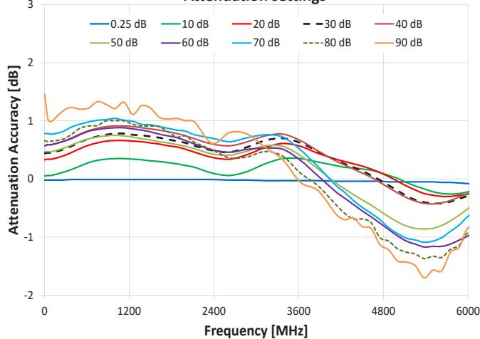
Attenuation Accuracy @ 0°C vs. Frequency over
