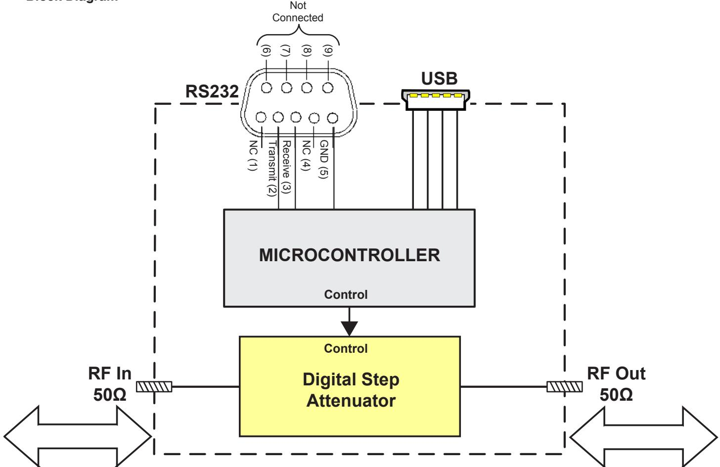
Simultaneous, bidirectional RF signal transmission with symmetrical performance
