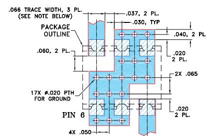
NOTES: 1. TRACE WIDTH IS SHOWN FOR ROGERS RO4350B WITH DIELECTRIC THICKNESS .030" ± .002"; COPPER: 1/2 OZ. EACH SIDE. FOR OTHER MATERIALS TRACE WIDTH MAY NEED TO BE MODIFIED. 2. BOTTOM SIDE OF THE PCB IS CONTINUOUS GROUND PLANE. DENOTES PCB COPPER LAYOUT WITH SMOBC (SOLDER MASK OVER BARE COPPER)
