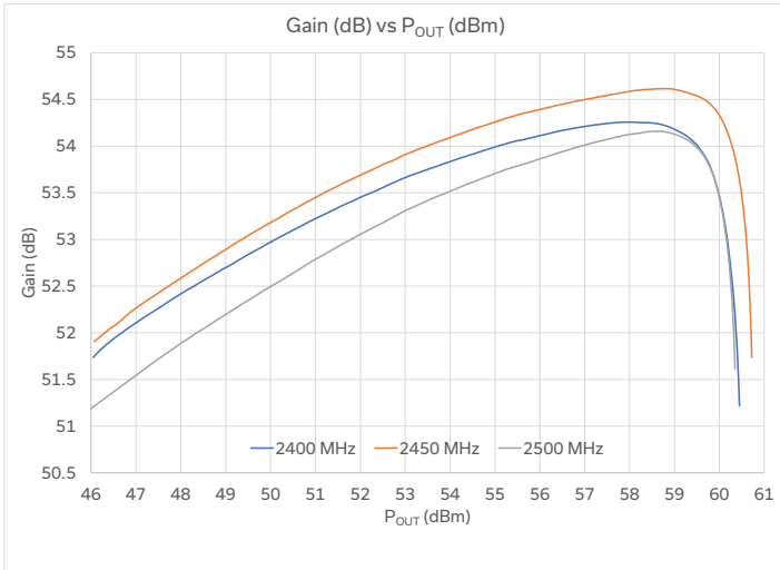
The RFS-2G42G51K0 is set to amplifier mode in the GUI. This is the AM-AM curve as a result of an external CW input.
