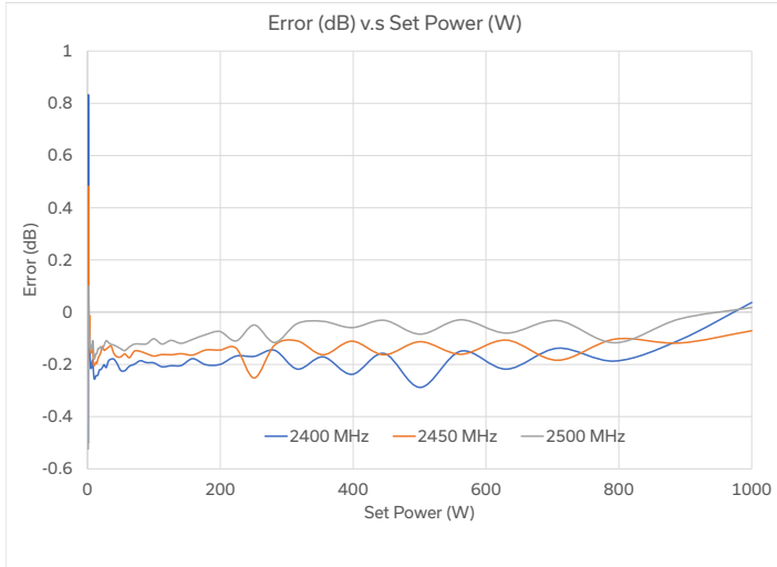
The RFS-2G42G51K0 is set to Normal Mode in the GUI. This is the error recorded in dB of the power measured by an external power meter to the power that was requested on the GUI front panel.
