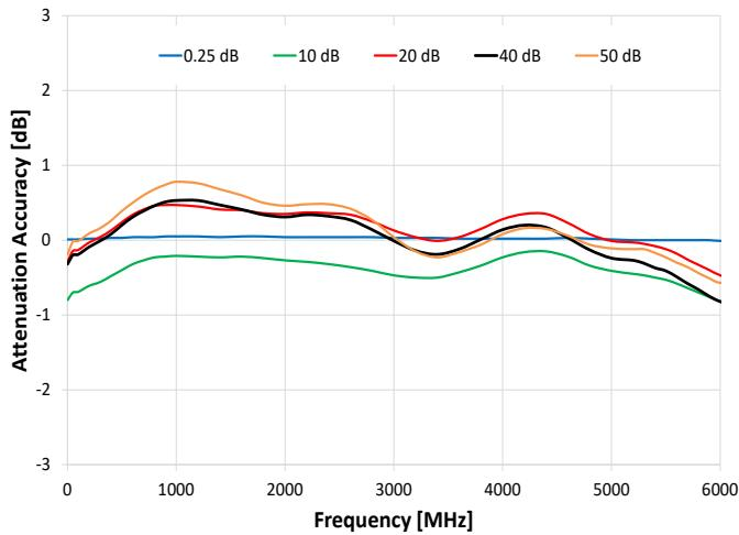
Attenuation Accuracy @ 0°C vs. Frequency
