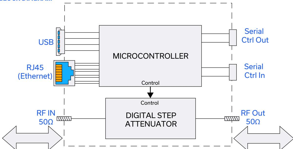
Simultaneous, bidirectional RF signal transmission with symmetrical performance
