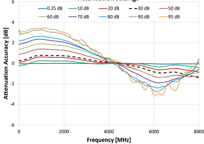
Attenuation Accuracy @ 30 dB vs. Frequency
