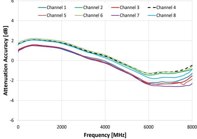
Attenuation Accuracy @ 50°C vs. Frequency over
