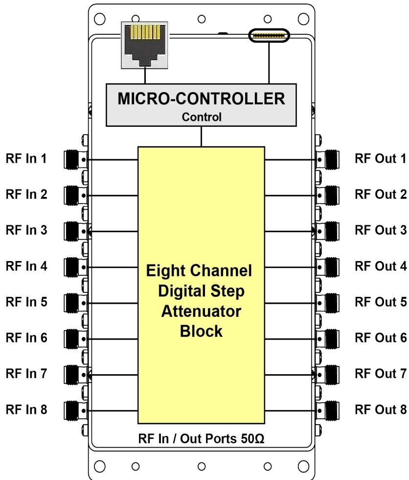
Simultaneous, bidirectional RF signal transmission with symmetrical performance
