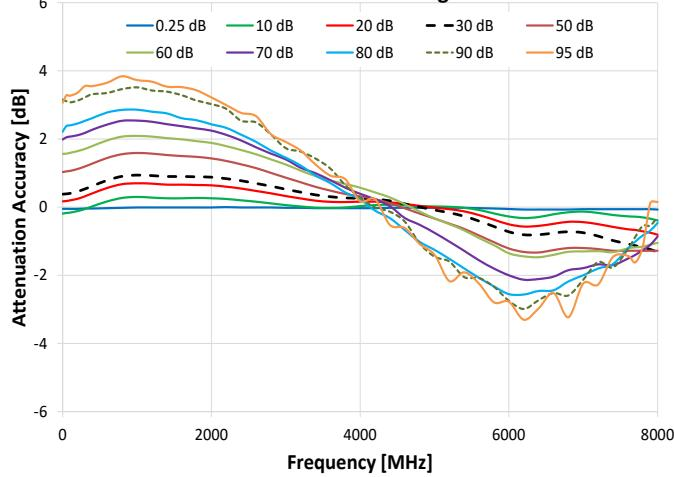
Attenuation Accuracy @ 60 dB vs. Frequency
