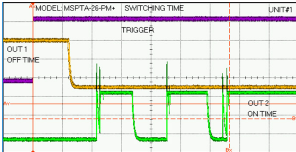
Switching from COM <> 1 to COM <>2 state: 13.30 ms
