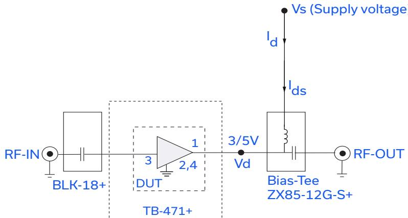
Fig 1. Block Diagram of Test Circuit used for characterization.
