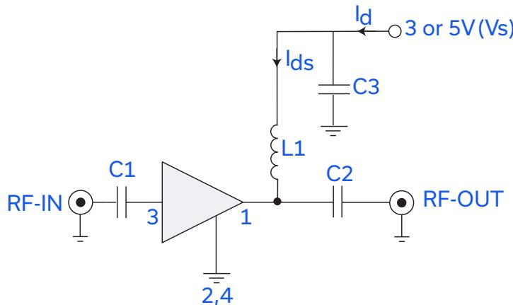
Fig 2. Recommended Application Circuit
