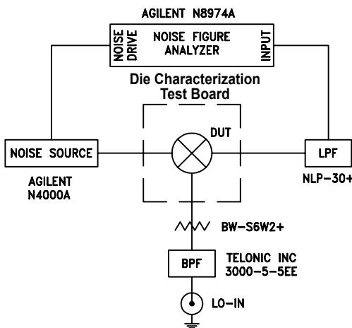
Figure 1B. Block Diagram of Test Circuit used for die characterization of Noise Figure
