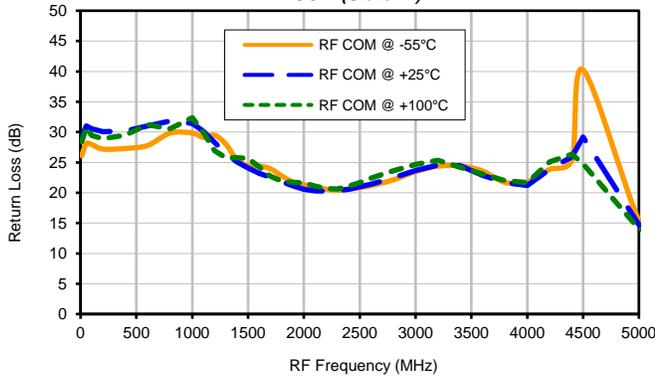
**RL @ VDD=+5V, VEE =-5V over Temperature**
