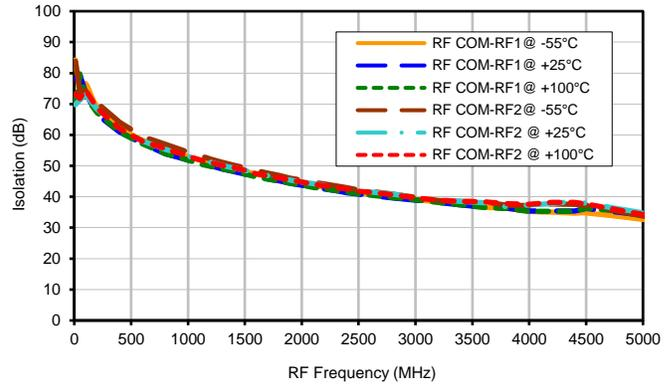
**Isolation @ VDD=+5V, VEE =-5V over Temperature**
