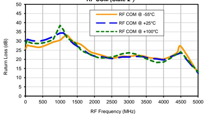
(1) Test data of Die packaged in industry standard, 3.25x3.25 mm, 8-lead MCLP package
