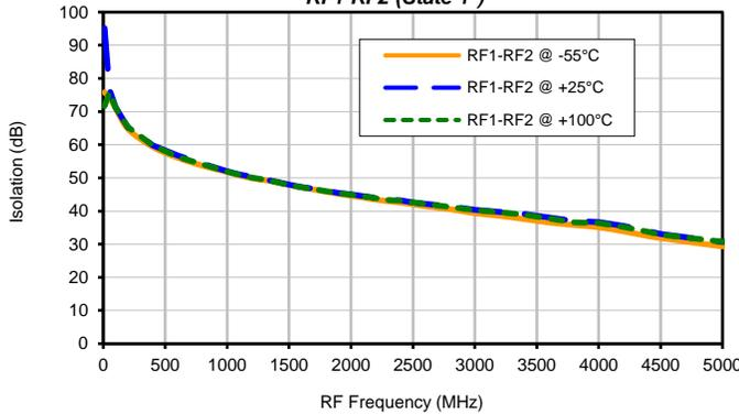
**Isolation @ VDD=+5V, VEE =-5V over Temperature**
