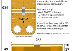
Section View of DIE on Carrier (units in mils)
