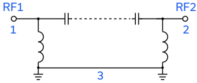
Figure 1. HFHKI-3100+ Functional Diagram
