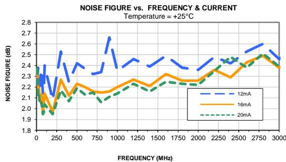
Note: Test data of Die packaged in industry standard SOT-89 package
