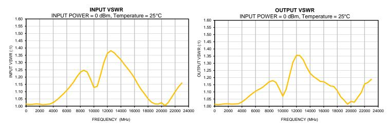
Note: Test data of Die packaged in industry standard 2x2mm 8-Lead MCLP Package
