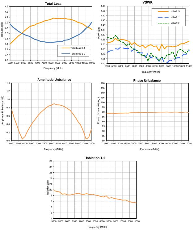
Note: Data tested on characterization test board TB-961-113+ in 4x4 mm MCLP package.
