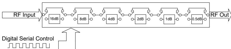
The DAT-31R5A-SP+ serial interface consists of 6 control bits that select the desired attenuation state, as shown in Table 1: Truth Table
