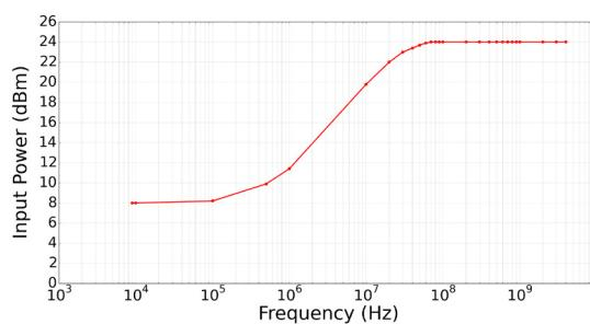
Figure 1. Max Input Operating Power vs Frequency
