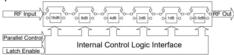
The DAT-31R5A-PP+ parallel interface consists of 6 control bits that select the desired attenuation state, as shown in Table 1: Truth Table
