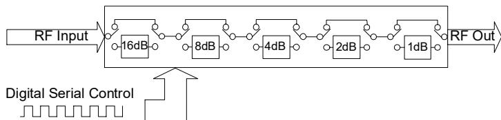
The DAT-31A-SP+ serial interface consists of 5 control bits that select the desired attenuation state, as shown in Table 1: Truth Table
