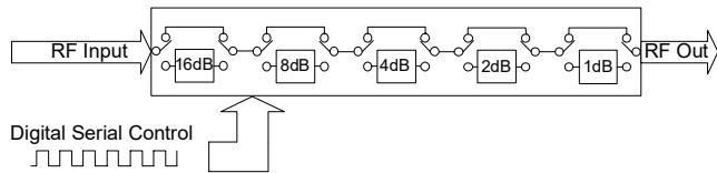
The DAT-3175A-SN+ serial interface consists of 5 control bits that select the desired attenuation state, as shown in Table 1: Truth Table
