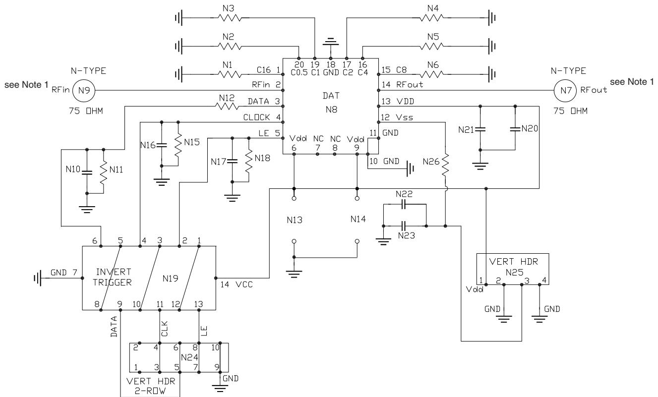
Note 1: Both RF ports must be held at 0VDC or DC blocked with an external series capacitor.
