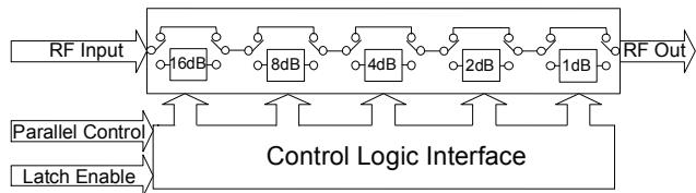
The DAT-3175A-PP+ parallel interface consists of 5 control bits that select the desired attenuation state, as shown in Table 1: Truth Table
