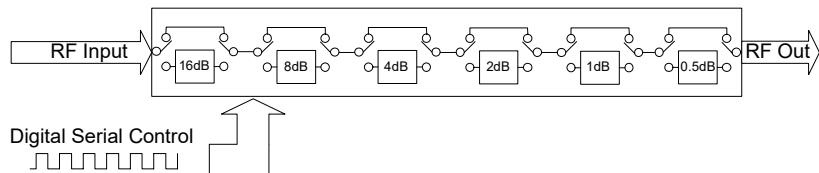
The DAT-31575A-SN+ Serial interface consists of 6 control bits that select the desired attenuation state, as shown in **Table 1: Truth Table**
