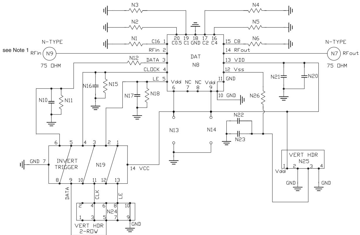
Note 1: Both RF ports must be held at 0VDC or DC blocked with an external series capacitor.
