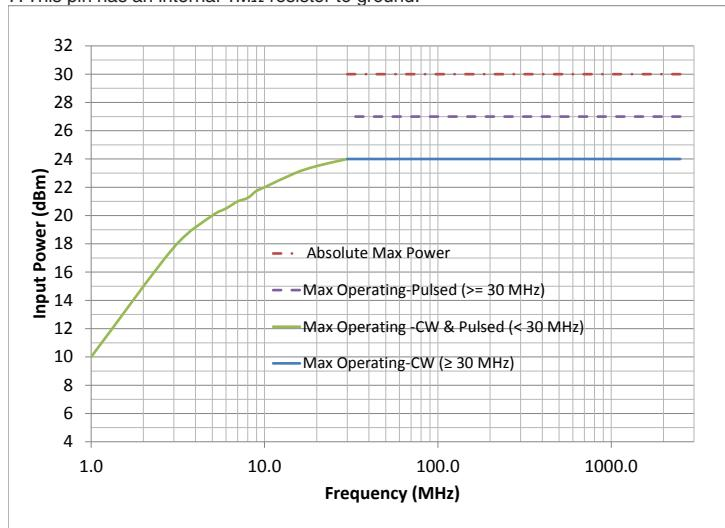
Figure 2. Max Input power vs. frequency.
