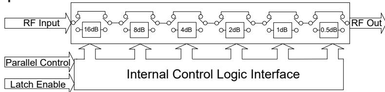
The DAT-31575A-PP+ parallel interface consists of 6 control bits that select the desired attenuation state, as shown in Table 1: Truth Table
