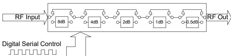
The DAT-15R5A-SP+ serial interface consists of 5 control bits that select the desired attenuation state, as shown in Table 1: Truth Table
