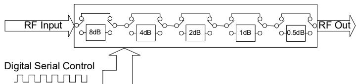
The DAT-15R5A-SN+ serial interface consists of 5 control bits that select the desired attenuation state, as shown in Table 1: Truth Table
