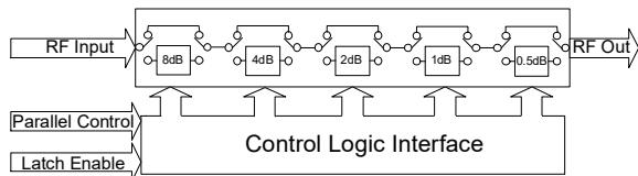
The DAT-15R5A-PN+ parallel interface consists of 5 control bits that select the desired attenuation state, as shown in Table 1: Truth Table
