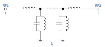
Figure 1. BFHKI-6751+ Functional Diagram
