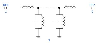
Figure 1. BFHKI-1252+ Functional Diagram
