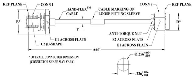
CUT OUT FOR SMA FEMALE BULKHEAD CONNECTOR
